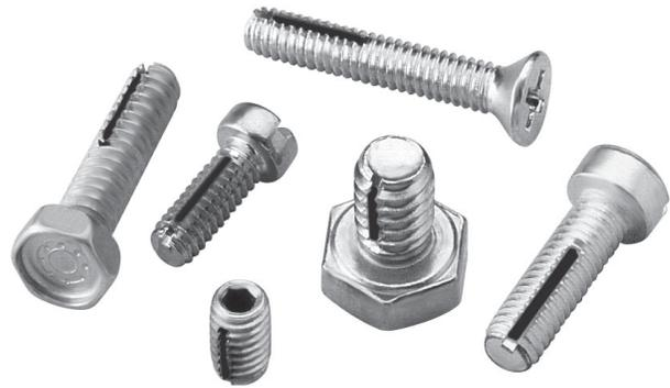
The Long-Lok strip fastener is a universally accepted, prevailing torque type self-locking fastener, with excellent vibration resistance. Over 35 years of use in thousands of proven applications attest to the wide acceptance of the Long-Lok strip. These fasteners are available in a wide range of sizes — from miniature eyeglass screws to fasteners for the heaviest of highway equipment.
